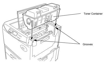
5. Check that the toner container is installed in the correct position, and push forcefully on the top of the toner container.
